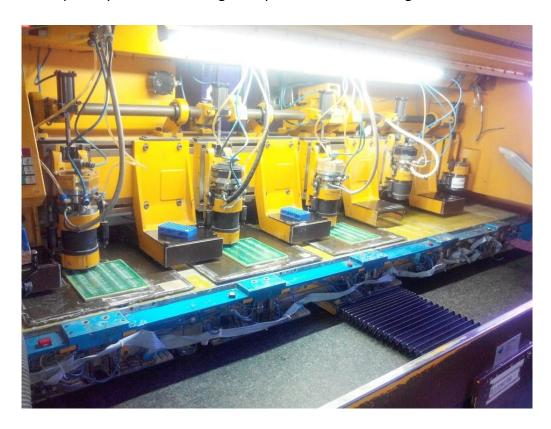
Posalux MULTIFOR 22 was equipped with Heidenhain special scales which were get damaged & customer machine became idle & did not able to utilize.
